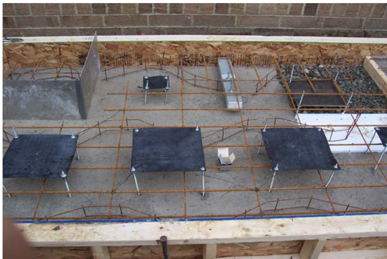
Figure 3 Test slab with purpose built defects
