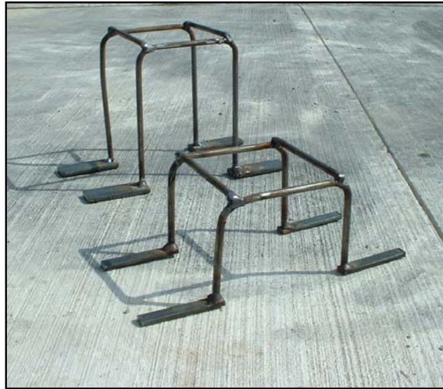
Figure 7 – Chairs for Sensor Installation 50 and 150mm below surface
