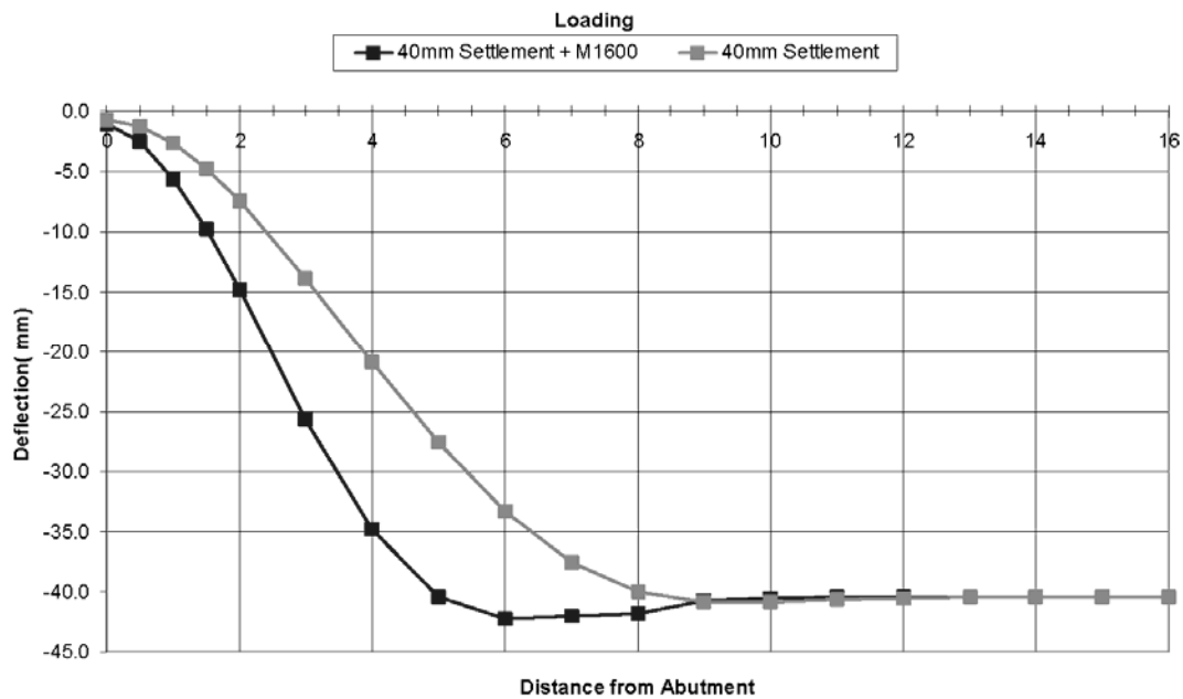
Figure 9: Approach Pavement Deflections
