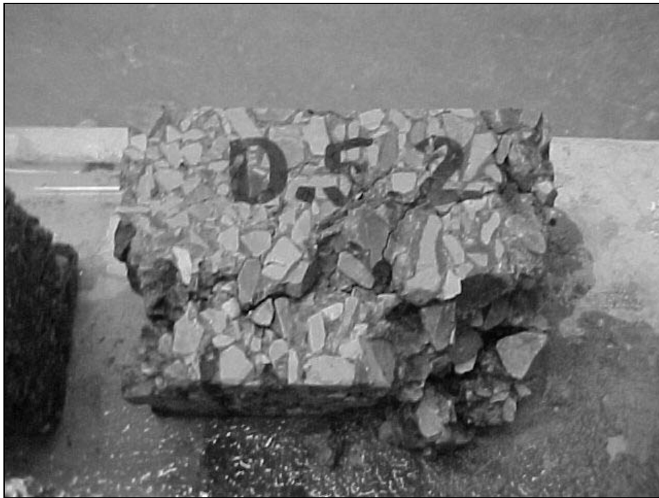
Figure 10. Specimen with freeze-thaw damage
