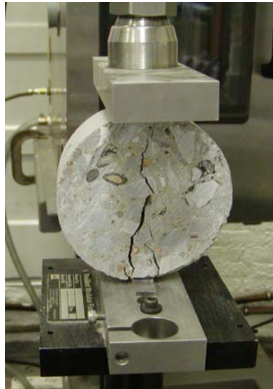
Figure 6. Split Tensile Strength Test Setup
