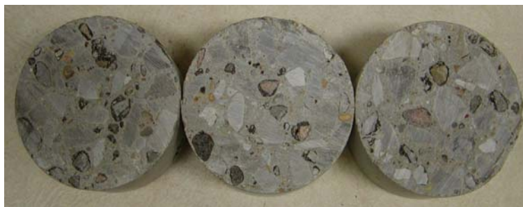
Figure 4. Split tensile strength test specimen
