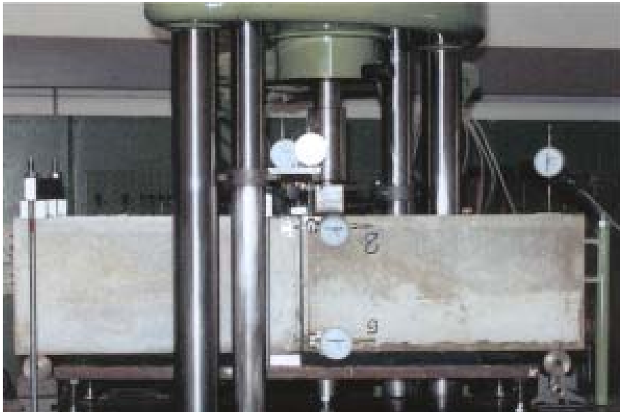
Figure 5. “Model beam” for the evaluation of the dowel’s joint effectiveness (comparative testing procedures)
