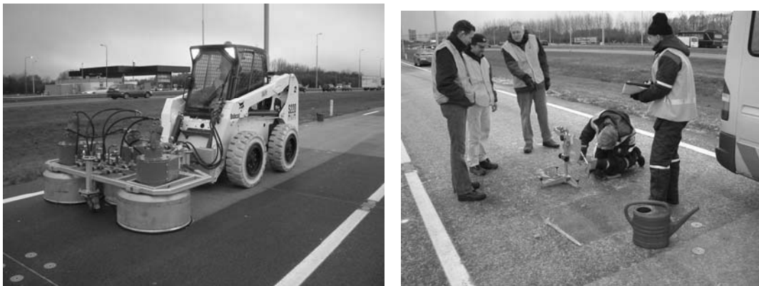
Figure 17. Sanding on the test section along the motorway A50 (left) and skid resistance measurement by means of the SRT device (right).
