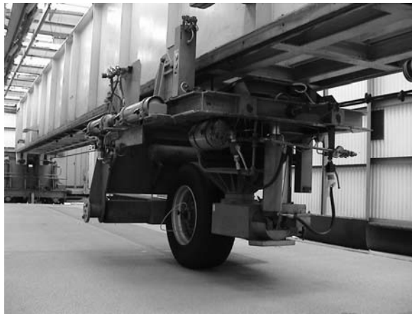
Figure 3. LINTRACK facility for Accelerated Pavement Testing.
