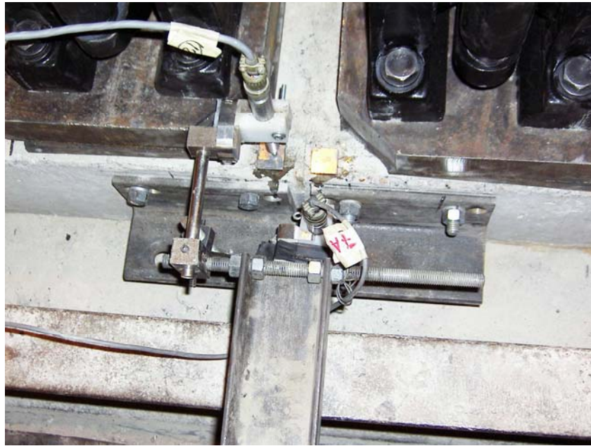
Figure 6. External LVDTs for measurement of corner and differential deflections.
