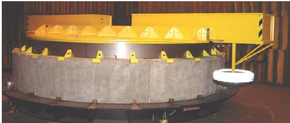
Figure 16. TPTA with the test specimens and tire mounted
