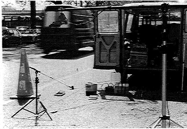
Figure 23: Measurement of absorption of porous surface by means of LCPC impulse method (French standard NF S 31089).
