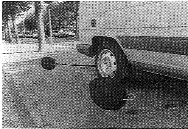
Figure 21: Rolling noise measurement: positioning of microphones in front and rear position in relation to the tire-pavement contact area. Height: 10cm from measured surfacing.
