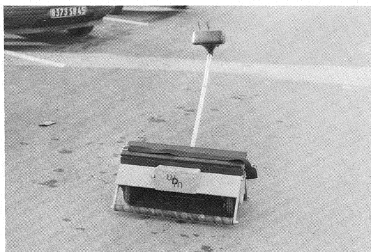
Figure 1 : Mini Texture Meter for measurements.
