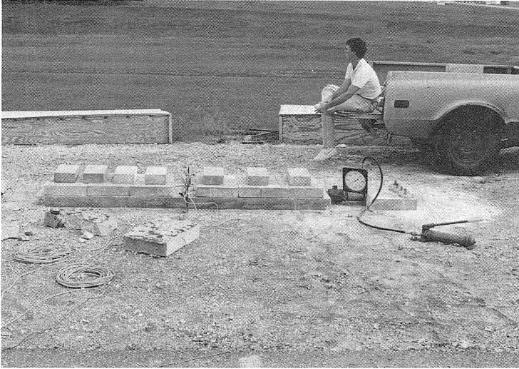
Fig 6. Eight-inch simulated slab for second push-off test in Austin, Texas (2).
